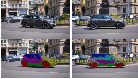
Figure 9: The effect of online adaptation on the representation of dynamic objects. As the object pose changes over time, newer visual words (denoted by gray and light-blue colors) are learned and added to the dictionary of visual words.
